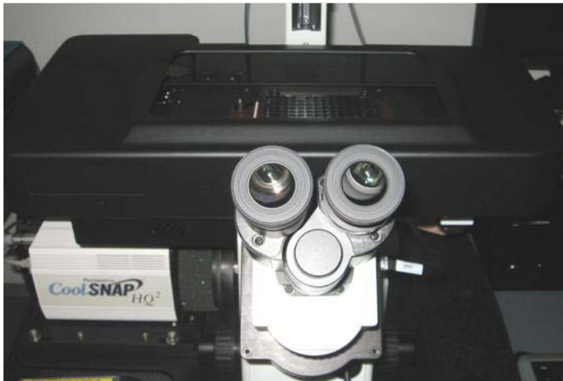
Microtiter Stage for DeltaVision Systems
