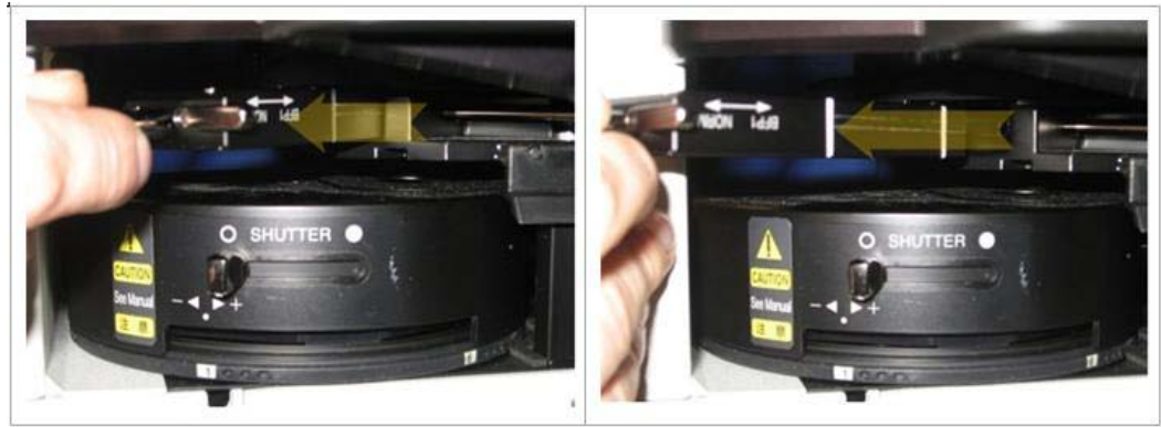
Removing the Principal Prism Slider from the Light Path
