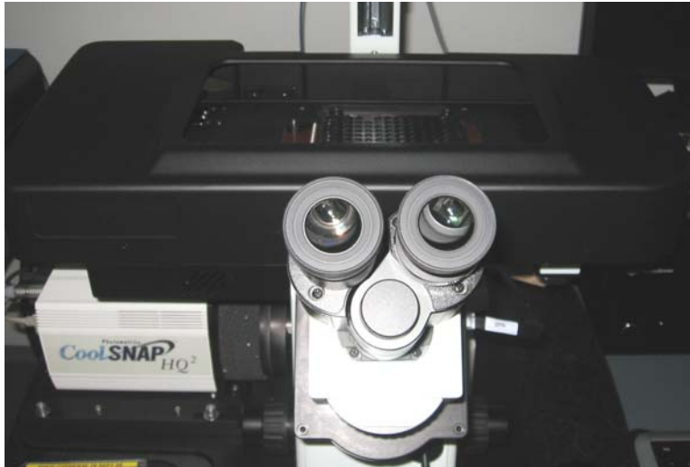
Microtiter Stage for DeltaVision Systems
