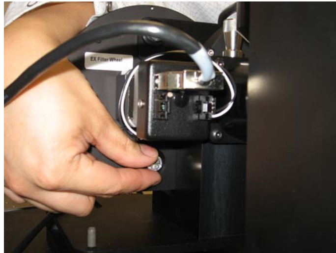
Loosening bottom thumb screw from filter wheel housing
