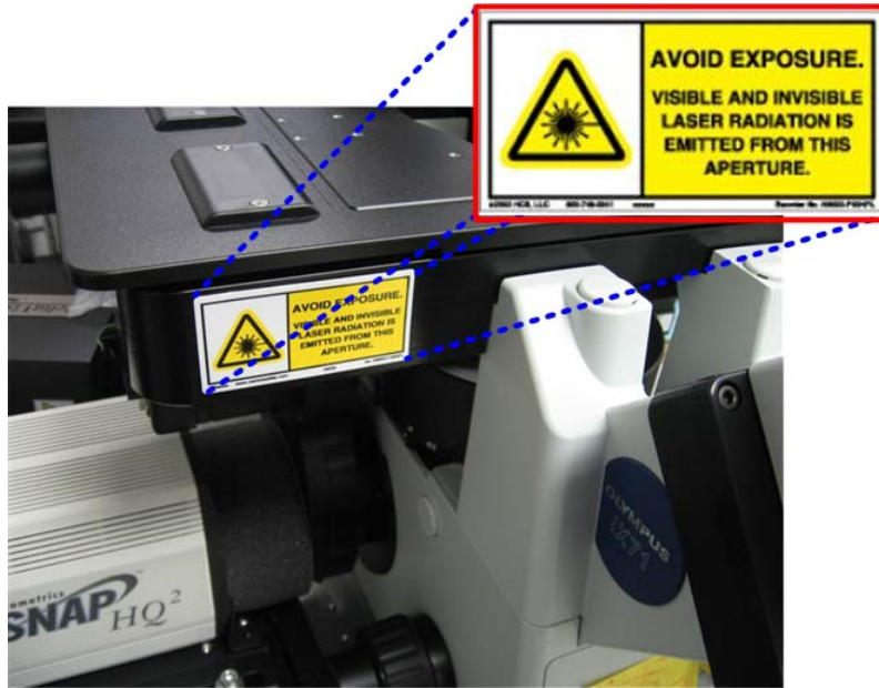
Laser Safety Label Location - DeltaVision Stage
