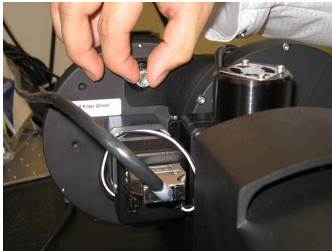
Loosening top thumb screw from filter wheel housing
