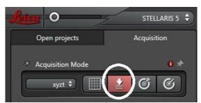
• Continuous mode: AFC always actively keeps the focus of the sample stable. Example application: when continuous medium injection happens during time course.
