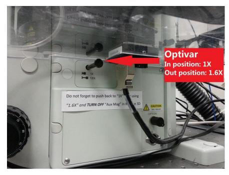
2. When using 1.6X auxiliary magnification, you need to turn on "Aux mag" in the Resolve3D software to match the actual scaling. This is very important, failing to turn it on, the size of
